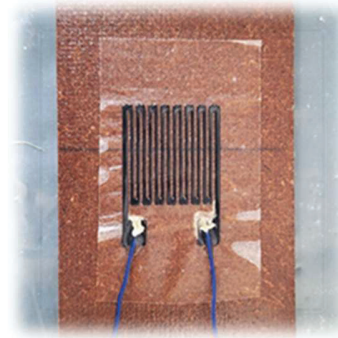
Fig. 3. 3D printed paper-based sensor, laminated with epoxy resins on a fiberboard.
