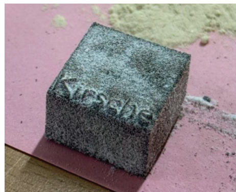
Fig. 2. Green part obtained by 3D binder jetting trials with the selected microcrystalline cellulose powder with PVP applied as powder binder.
